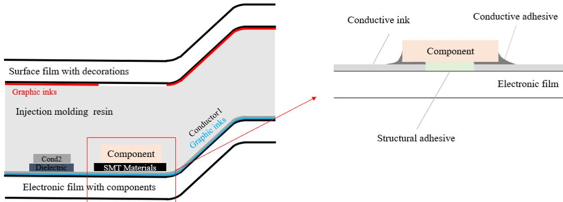
**Figure 4 - Typical material stack in structural electronics**
