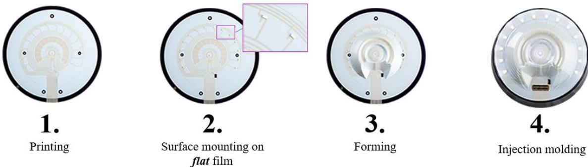
**Figure 3 - Core manufacturing processes for structural electronics**
