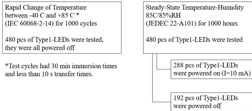
**Figure 7 - Summary of tests and sample sizes in Type1-LED reliability testing**
