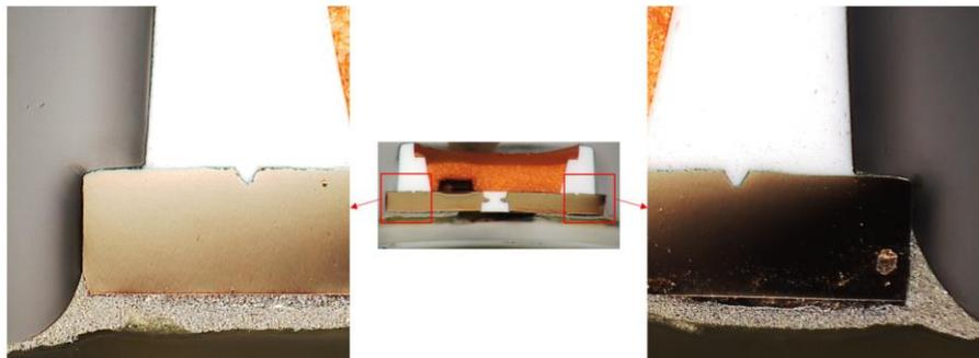
**Figure 8 – Cross-section shows slight bending of component base and partial delamination of conductive adhesive.**
