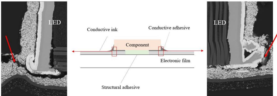
**Figure 12 - SEM-images of the cross-section show fracture in the conductive adhesive used for surface mounting.**
