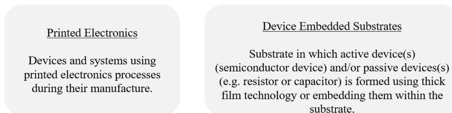
**Figure 13 - Definitions for Printed Electronics and for Device Embedded Substrates**
