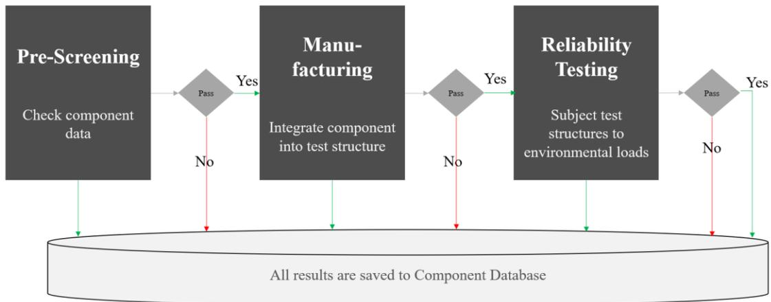
**Figure 5 - Component certification process flow.**
