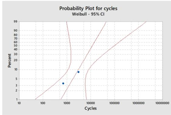
**Figure 11 - Extended reliability testing failures in Weibull-distribution**
