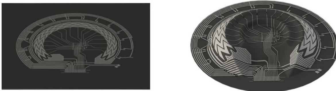
Figure 3 - Illustration on left shows two-dimensional IMSE film after printing. Illustration on right shows three-dimensional film after thermoforming (and cutting).
