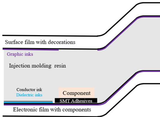
**Figure 4: Illustration of a material stack in a 2-film design**
