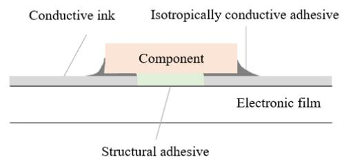
**Figure 7: TactoTek uses isotropically conductive and structural adhesives for surface mounting**
