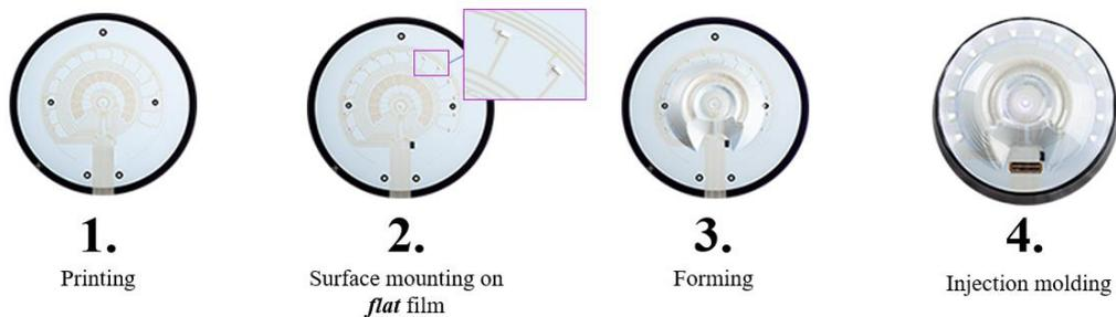
Figure 3: Core manufacturing processes for IMSE
