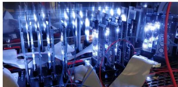
**Figure 10: Photo of the MSPs that were powered on during Steady-State Temperature-Humidity (85/85) testing**
