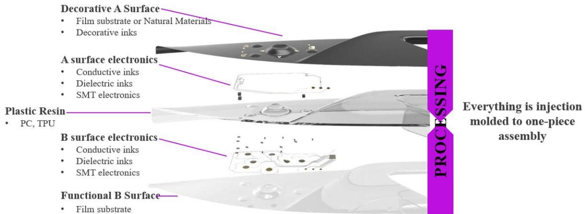
Figure 2: Illustration of materials in IMSE design.
