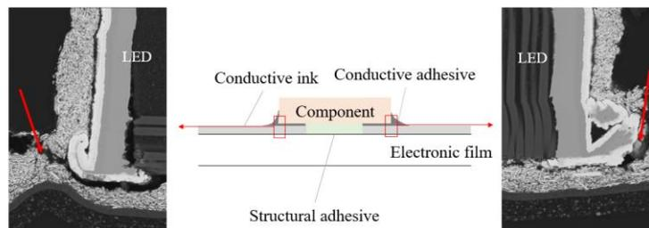
**Figure 14: SEM-images of the cross-section show fracture in the conductive adhesive**
