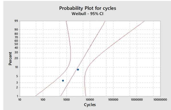
**Figure 13: Extended reliability testing failures in Weibull-distribution**
