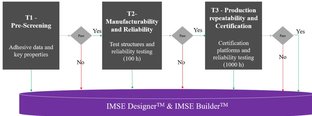
**Figure 8: Surface mounting adhesive certification process**
