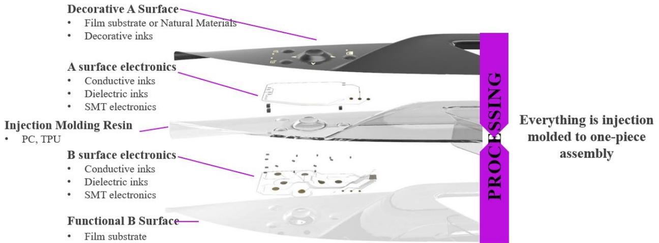
**Figure 2. Illustration of materials in structural electronics design**
