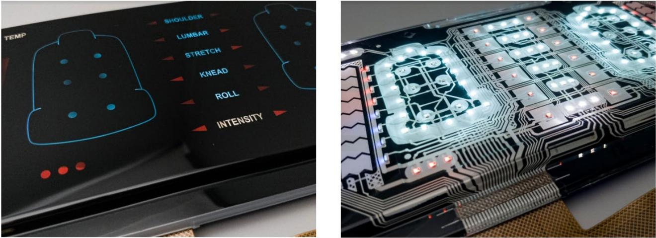
**Figure 5. On the left: the back-seat-control-panel. On the right: the same panel with clear A-film and injection molding resin so that electric components are visible.**
