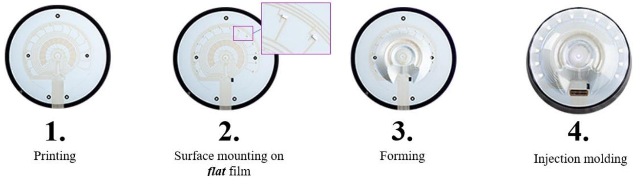
**Figure 4. Core manufacturing processes for structural electronics**
