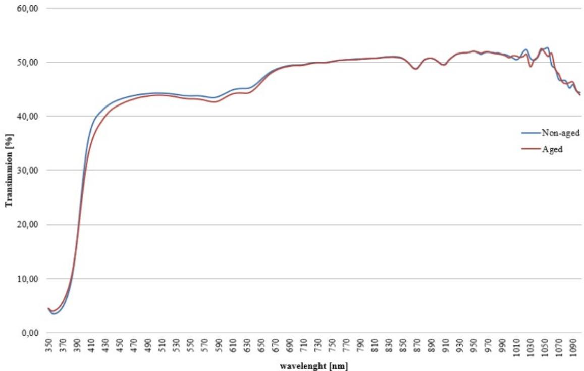
**Figure 7. Transmission measurements for injection molding resin material, sample thickness is 3 mm<sup>3</sup>. The transmission spectrum is similar for non-aged and aged samples. Table 2 shows the relevant wavelengths for blue, red and white LEDs.**
