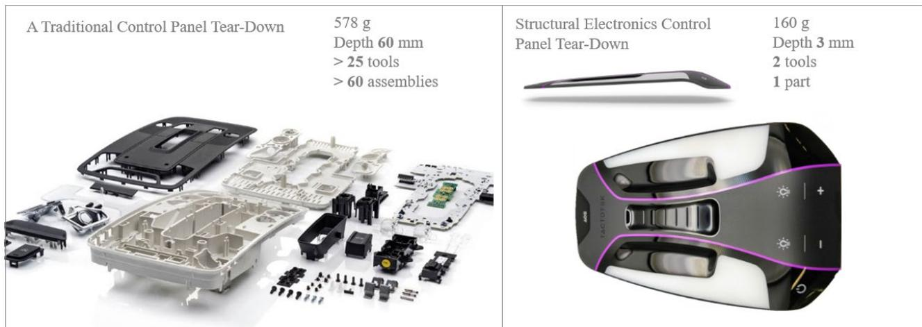
**Figure 1. Structural electronics control panel design demonstrates 70% reduction in weight and 90% reduction in thickness when compared with conventional multi-part assembly.**
