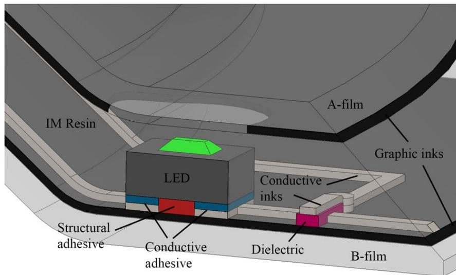
**Figure 3. Illustration of a material stack in two-film design.**
